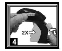
Close the label compartment door. Squeeze the handle two more times to continue feeding the tape through the unit.
