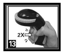
Firmly squeeze the handle to advance the tape without embossing any characters.
