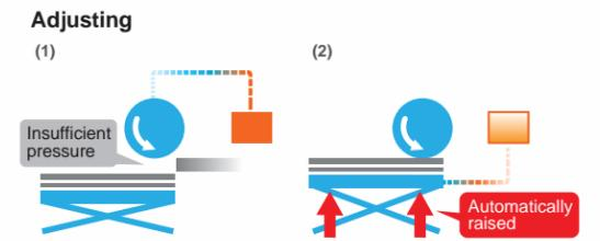
The sensors detect when the paper feed is not correct due to insufficient pressure.
