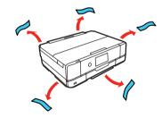
2 Lift up the scanner unit. Remove all protective materials from inside the product.
